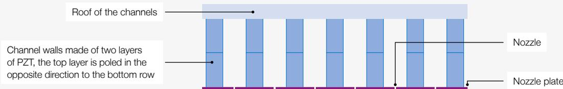
The diagram above shows the ink channels in a ‘neutral’ state. i.e. inactive and non-firing.
