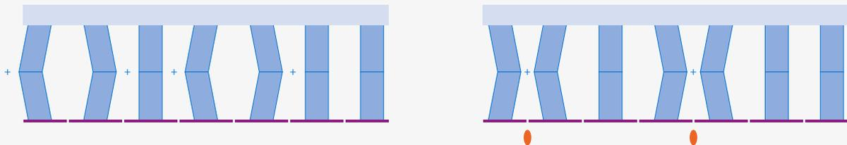
The diagrams above show what happens when a voltage is applied to the channel walls. As there are two layers of PZT which are poled in the opposite direction, when a voltage is applied, the PZT walls move in a chevron-shaped motion. As the walls move, acoustic waves are generated.
